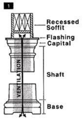
1. Adequate ventilation is a necessity in the installation of wood columns. It must be provided for at the top of the column by a recessed soffit and at the bottom by the precut openings in the plinth.
