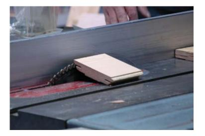
NOTE: To use corners on material less than 3/4" thick, simply glue a wood strip or cleat to the panel edge prior to shaping.
