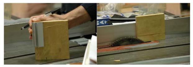
2. To make the inside cut, adjust the blade 3/8" from the fence, with the finish side against the fence. This cut is critical. Any variance will not allow a proper fit for the extrusion.
