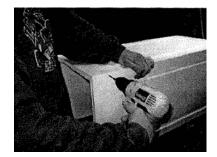
**6.** Screw or pin-nail the three panels together into one unit.
