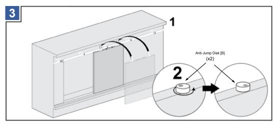
Attach the doors to the rail and lock the anti-jump disks [B] into position. Doors should be routed beforehand if using the routed door guide [C].
