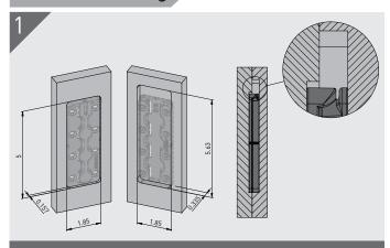
**Part Rebate** - each substrate mounting face is rebating as shown. Ensure sufficient screw embedment in substrate.
