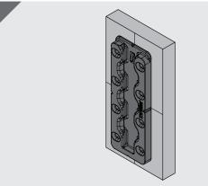
Flush mounting requires no additional preparation. Line the notches in each component (Hook shown here) with the center lines. Mark-Out Template can also be used.
