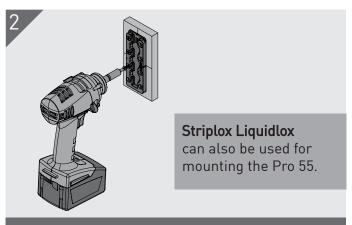
Hold the component in place and fasten to the substrate with 8 x 8G screws. Repeat for matching component. Ensure sufficient screw embedment in substrate.
