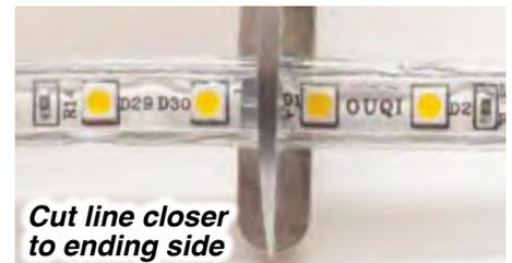
Helpful Hint: The tendency is to cut right in the middle or straight in half instead, it is recommended to cut closer to the finished end where you will attach an end cap. This allows more room to attach the power cord to the next section.
