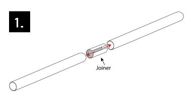
Use the joiner to join the two lengths of rail together. **NOTE:** For four foot kit, begin with step 2.
