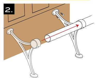
Slide the combination brackets onto the rail and secure them to the bar with the provided screws.
