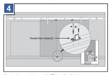
If using the routed door guide [C], install at this time.
