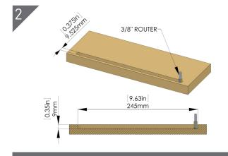
Use a 9.525mm (3/8") router bit to cut a slot in both substrates to correct length. Depth needs to be 9mm.
