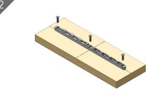
Place Megalox onto surface in position and pilot drill screw position use 3x 8G countersunk screws or Euro screws.
