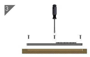
Place the 1st Megalox into slot ensure flush with substrate. Pilot drill screw position, use x 3 8G countersunk screws, Euro screws or simply glue into position using Liquidlox.
