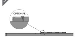
Megalox is either permanent or reuseable, simply remove locking tab using blade or sander to disassemble.
