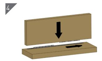
Complete the installation by sliding fully to lock up position.
