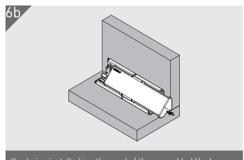
Key being installed in other end of the assembled Hooks.
