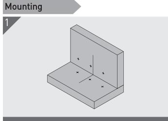
Mark center line on both substrates. The 90D 98 works on box joints (shown), t-section and mitered joints. Mark mounting screw centre points by measuring or with the aid of the Mark-Out Template.
