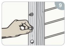
Snap on decorative End Caps over the exposed ends of the Quick-Connect®SS fittings and Snug-Grip® Washer Nuts.
