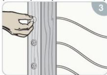
Insert the Threaded Terminal into one end termination post and secure with a Snug-Grip® Washer Nut.
