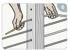
Lace the free end of the cable through the intermediate posts. We recommend using our lacing needle for smoother threading through post holes and to prevent cable strands from catching on the sides of the post holes during installation.
