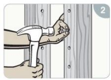
Insert Protector Sleeves (wood posts) or Grommets/Isolation Bushings (metal posts) at necessary locations.
