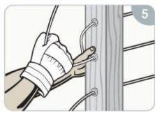
Pull the cable through the Quick-Connect®SS fitting to remove the excess slack in the line.
