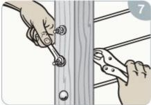
Tighten the Snug-Grip® Washer Nuts to adjust the final tension in the line.
