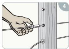
Lace the free end of the cable through the remaining posts and slide on a Quick-Connect®SS fitting.
