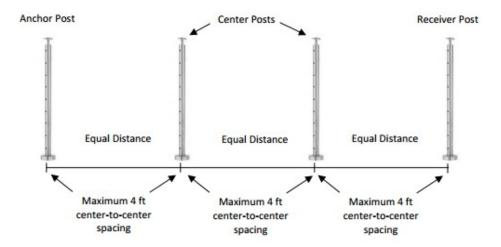
Mount posts to the floor or fascia. Use lag bolts for mounting to wood, machine screws
