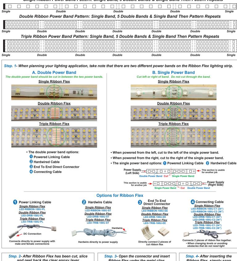
and peel back the clear epoxy layer exposing the conductive ends.
