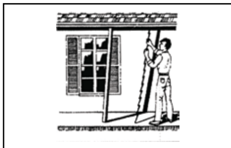
Before assembly, measure opening. Cut column staves 1/8" longer with a hacksaw.
