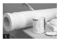
**1**. All interior columns, caps and bases must be primed with one (1) coat of primer and then painted with one (1) coat of paint. NOTE: While both latex and oil-based products may be used for interior applications, oil-based products have better adhesion. Follow the paint manufacturer's instructions for best results. Wood caps & bases are not vented and should not be used for exterior use.
