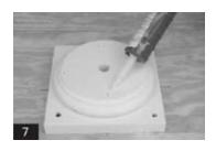
7. Apply a bead of paintable silicone sealant around the top perimeter of the base and place the shaft on top of the base.
