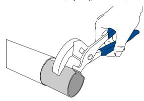
**TIP**: Use a wrench to crimp the joiner in order for it to fit inside the rail.
