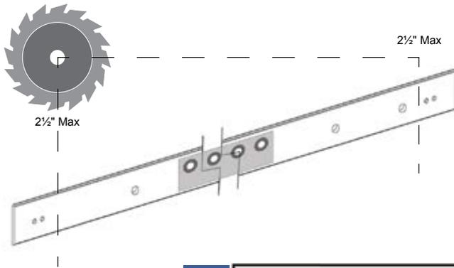
The rail can be trimmed if necessary using a band saw or hacksaw. Use blades suitable for iron or stainless steel depending on your rail.
