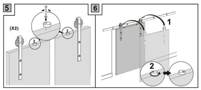
Attach the anti-jump disks to the tops of the door.
