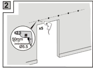
Using a power drill with a 50mm drill bit, drill holes into wall blocking. Attach the wall portion of the brackets at this time.
