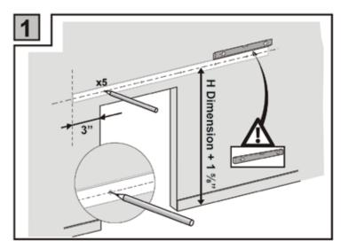
Find the centerline of the track. Using a level, mark a horizontal line twice the door width long. Mark the bracket screw locations into the wall blocking.
