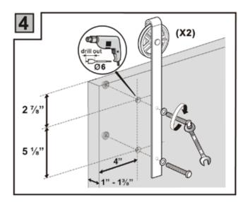
Drill out holes in the door using a 6mm routing drill bit as pictured. The bottom of the door should be routed at this time in order to accept the floor guide.
