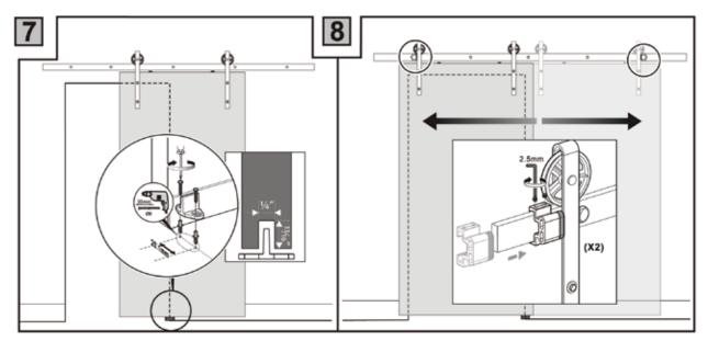
Plumb the door and mark the positions of the floor guides. Mount the floor guides to the floor.
