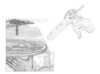
Apply a ¼" bead of premium polyurethane adhesive all around the back of the medallion. While applying, make sure the medallion's back is facing up. Press the medallion against the ceiling. Wipe off any excess adhesive with a damp rag or sponge before it can harden. Use finishing nails if needed. If the ceiling is uneven, you can use painters caulk to fill in any gaps. Touch up paint can be used if needed.
