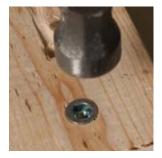
Use a hammer to tap a 5/16-18" insert nut into the drilled hole.
