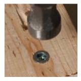
Replace with a  $\frac{5}{6}$  -18" threaded insert nut. Use a hammer to tap in the insert nut.
