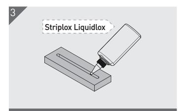
Apply Striplox Liquidlox 15 second cure adhesive to both sides of the slot in each substrate. Visit outwater.com or call 1-800-631-8375 to find out more about Striplox Liquidlox and Mark-Out Template.
