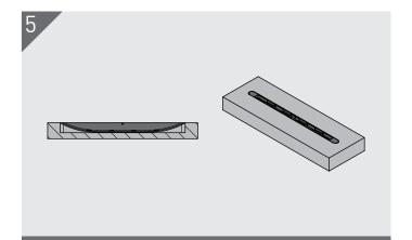
After glue is applied, insert Hook and Key into slot until flush with substrate. Allow to dry as per glue manufactures instructions.
