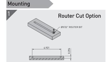
Use a Ø9/32" router bit to cut a slot in both substrates where the Hook and Key of the Mini 120 is to be mounted. Depth needs to be 0.394" for each.
