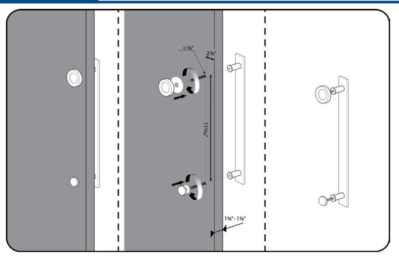
Drill holes into the door with a 3/8" drill bit. Holes should be spaced 11-13/16" apart and 2-3/8" from the edge of the door. Refer to the above diagram to install the pull.
