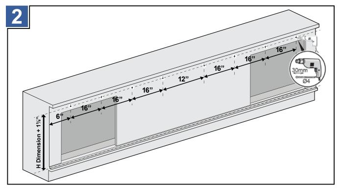
Using a power drill with a 4mm drill bit, drill holes as indicated.
