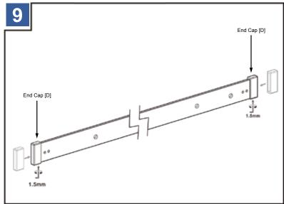
Once cut, add the end caps [D] to the ends of the rail and secure with a set screw.
