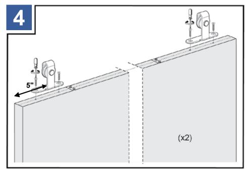
Drill holes into the doors as indicated. Attach the door rollers [A].
