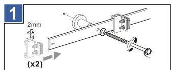
Before beginning installation, attach the door stops [C] to both rails [M].
