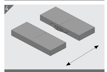
Position both surfaces together aligned and move together (180 degree joint).
