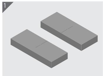
Mark out position on both surfaces to align.
