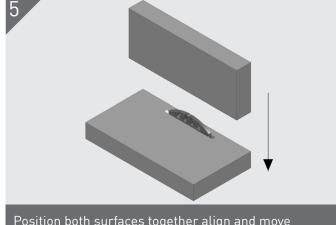
Position both surfaces together align and move together (90 degree joint).
