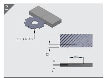
Set depth stop to #20 on Biscuit cutter and plunge in on centreline position or cut position with router using 4mm bit.
