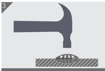
Position Biscuit at centreline and knock in with hammer, unique grips will hold in place (no glue required). Glue may be used (CA). Glue will travel into void areas.
