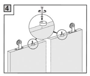
Attach the anti-jump disks to the tops of the door.
