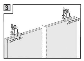
Drill holes in the top of the door 3-15/16" from the edge as pictured to accommodate the door rollers. The bottom of the door should be routed at this time in order to accept the floor guide.
