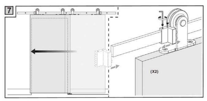
Adjust the door stops accordingly using the provided Allen key.
