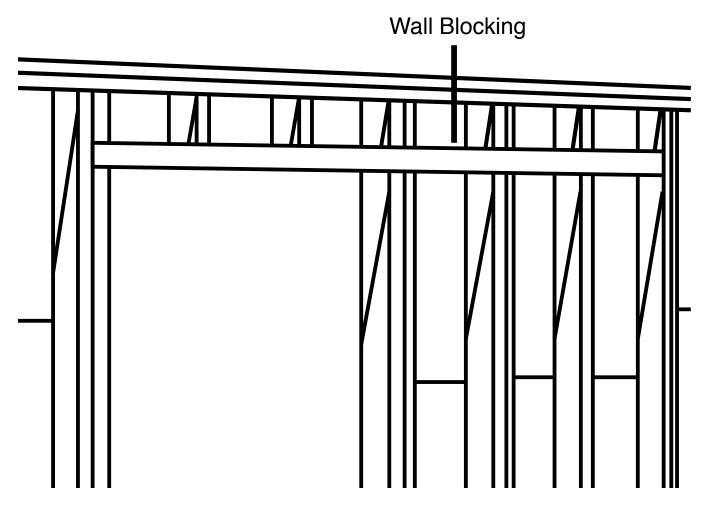
Brackets must be secured into wall blocking.
